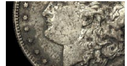
Corrosion, as shown on this Morgan dollar, will result in a "Details Grade" designation.
