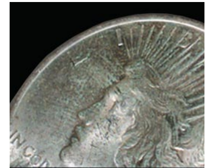
This Peace dollar has a layer of PVC residue that is easily observed. Note the "off" color of light green haze on the coin's surface.
